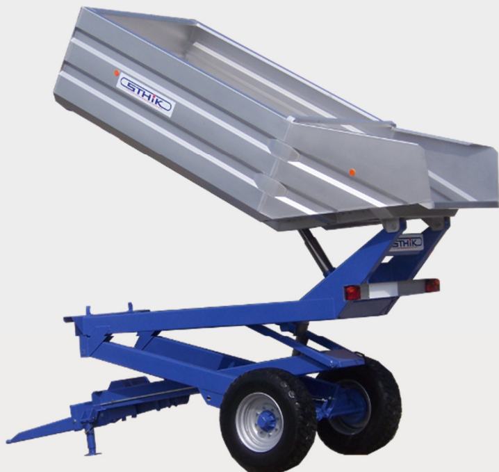
SB : Lifting & Tipping
