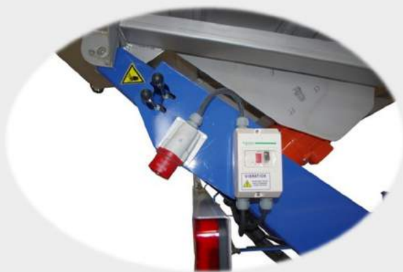
Dual Control : Tipping and lifting are controlled from the trailer
