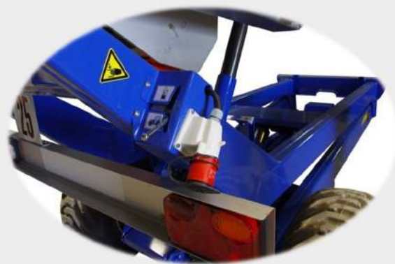
Dual Hydraulic Circuit for tipping bin with Power Pack or tractor
